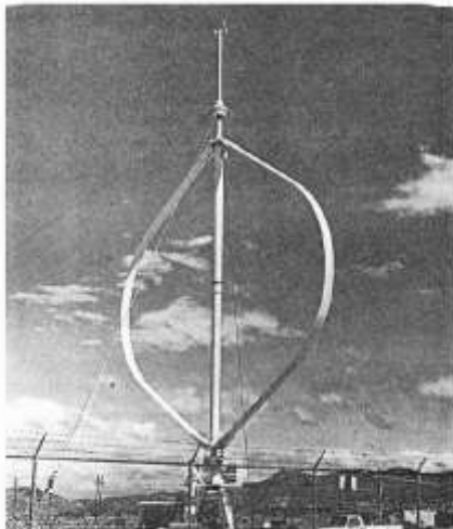
Sandia Laboratories 17-m Darrieus, rated at 60 kW in a 12.5-m/s wind.
